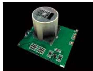
Tall component in SMT process
