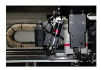
The right laser, whether CO2, UV or fiber laser, can be integrated for every application. A variety of materials such as solder resist, metals, plastics or ceramics can be marked.
